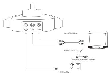
Figure 7. Connection diagram
